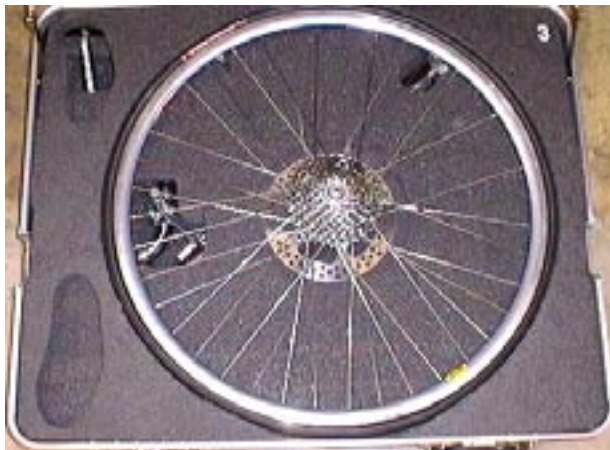
Layer #3: Rear wheel with cog set facing upward
