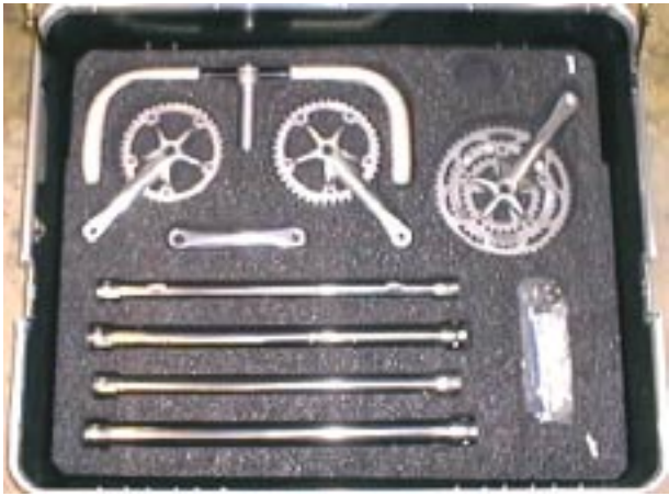
Layer #1: Stoker bar & stem, cranks, rear top tube, rear lateral tube, bottom tube(s)
