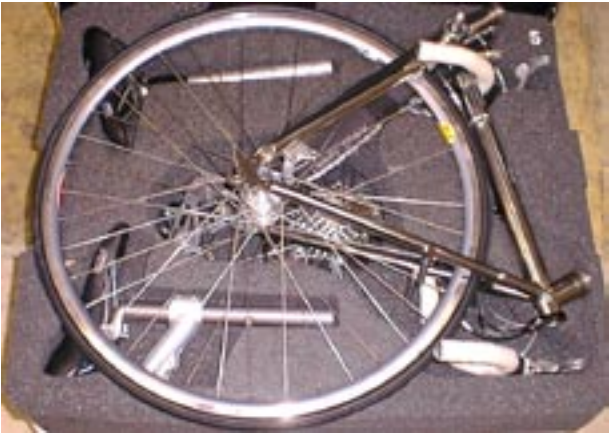
Layer #5: Step 2 Place rear triangle with front wheel tucked in above saddles and seatposts.
